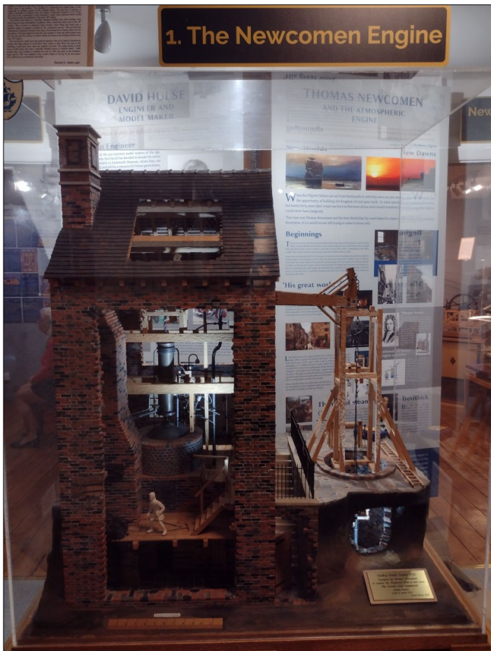
1/16 th scale model of Newcomen's 'Dudley Castle' engine. Image courtesy of Geoff Wallis.
