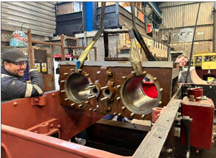
Installing the new cylinder block on Hudswell Clarke locomotive.
