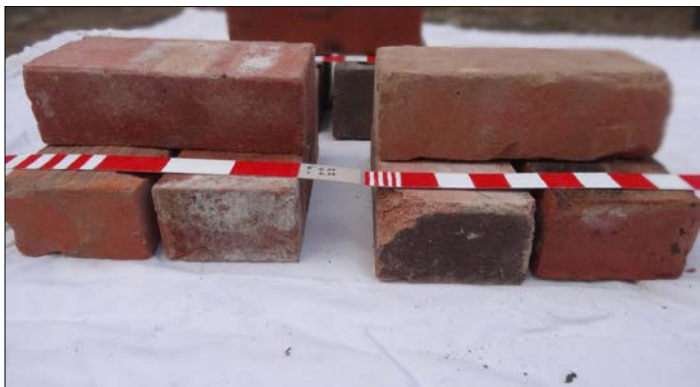
Fig 3 (Below): Imperial and metric bricks. Fig 4 (Bottom): 9in x 4 1 / 2 in bricks. Image copyright John McGuiness.
