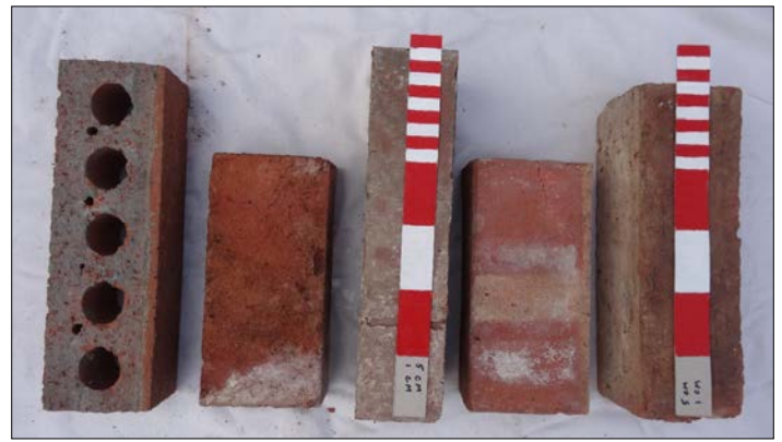
Fig 5: A variety of metric brick sizes alongside standard flettons.
