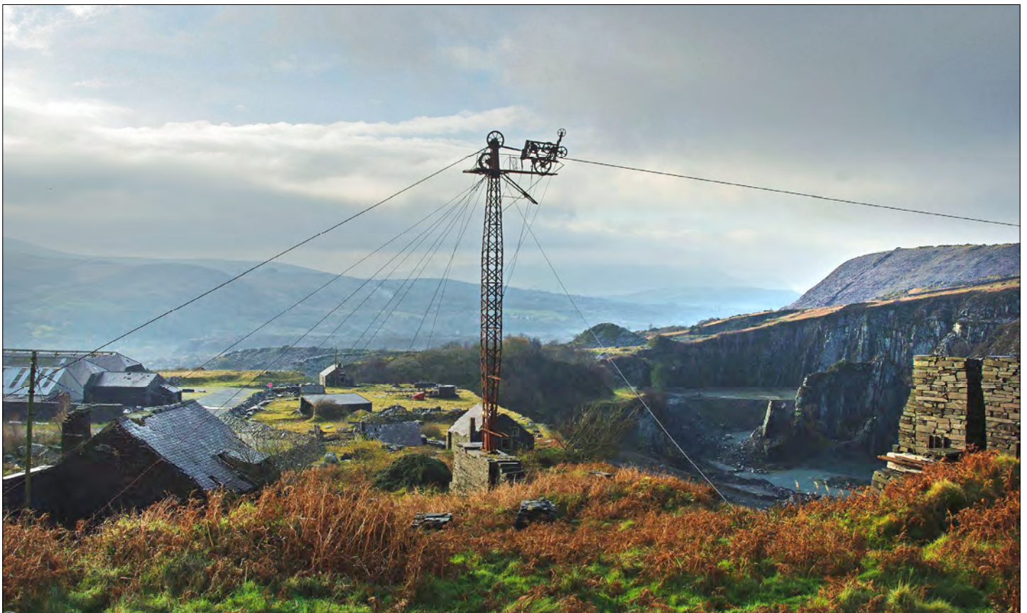
Nantlle Valley Slate Quarry Landscape - 'Blondin' ropeway, Pen yr Orsedd Slate Quarry. Image copyright Dave Hopewell, Gwynedd Archaeological Trust.
