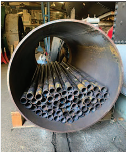
A new barrel and set of 55 seamless and swaged combustion gas boiler tubes.
