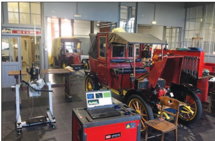
Fig 4. Acoustic emission test performed on a Renault AG1. © HE Arc CR 2019
