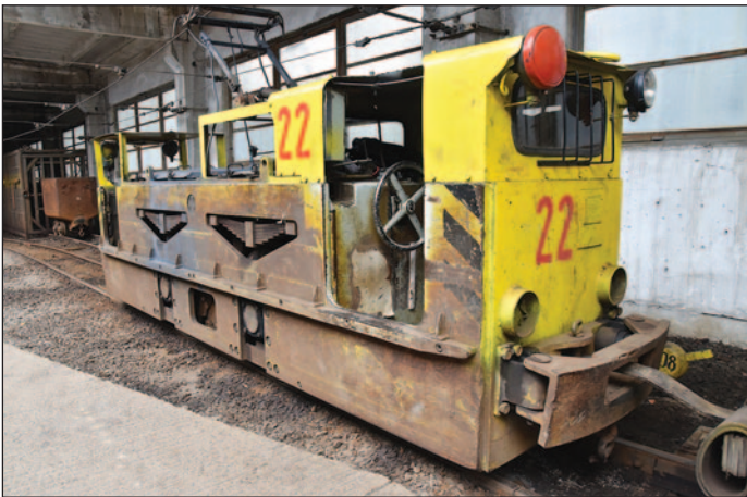
Electric trolley locomotive at the main train platform, Cigel' Brown coal mine - Baňa Cigel', Sebedražie, Slovakia
