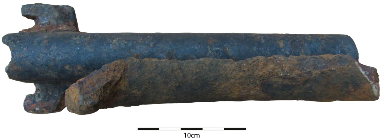
Figure 19. A single flange from a double-flanged wheel, resting upon a rail and showing the split down the rim's centre.
