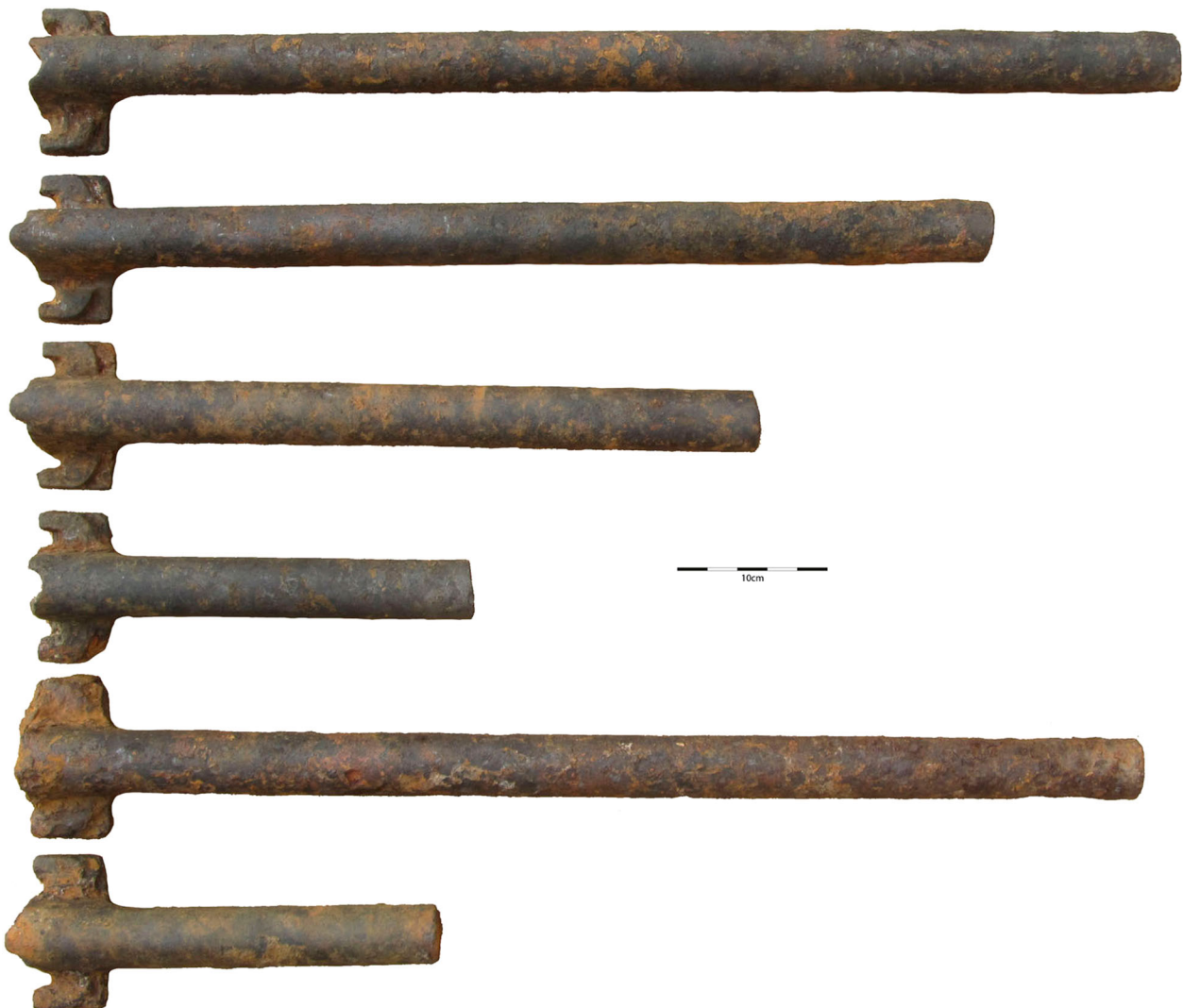
Figure 12. Rail specimens as viewed from above. The upper four examples are shallow-belly rails, and the lower two are deep-belly rails.
