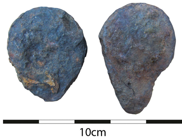
Figure 9. The 'egg-shaped' cross-section of the Congleton rails. Both of these rails broke at a similar length, comparing shallow-belly (left) and deep-belly (right).
