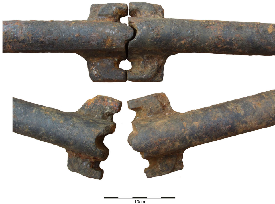
Figure 10. Details of the feet cast at either end of the Congleton rails, showing the lugs and the holes used for spiking them down.
