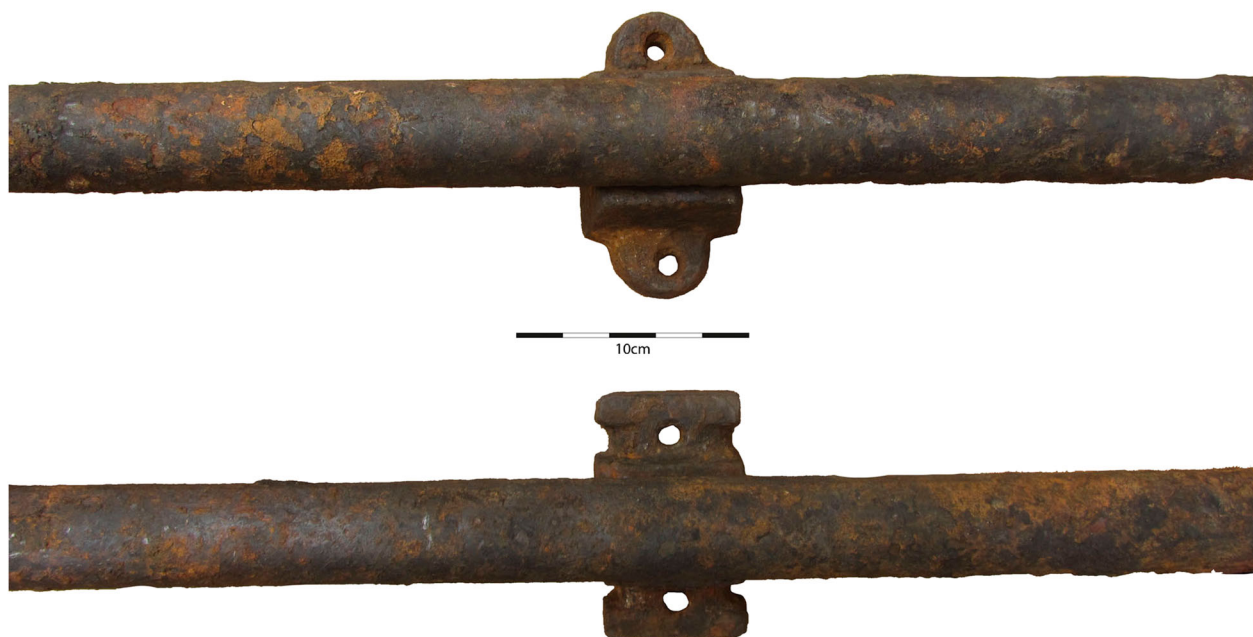
Figure 14. Saddles in use for supporting rails, with a plain saddle (above) and a lugged saddle (below).
