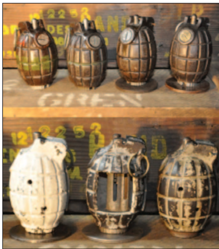
4 inert JPS service grenades and below, 3 practice grenades, (with holes to avoid mistakes) the middle one sectioned at Primet foundry for instruction, the left hand one for rifle launching and that on the right for throwing.
