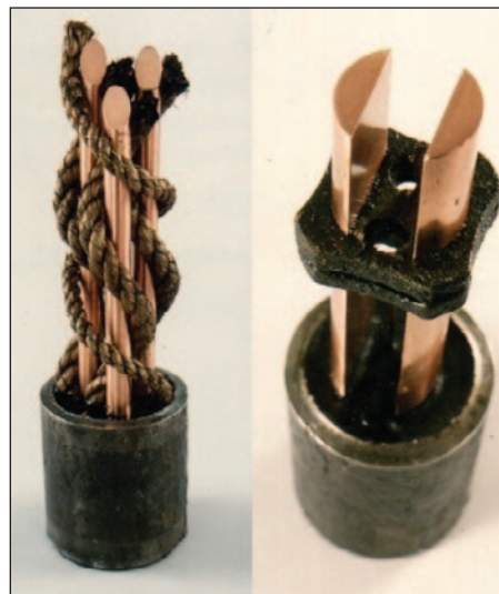
Cut-away examples of the 3-core (1892) and 2-core (1884) Edison Street Tubes recovered in 1992, showing the internal construction
