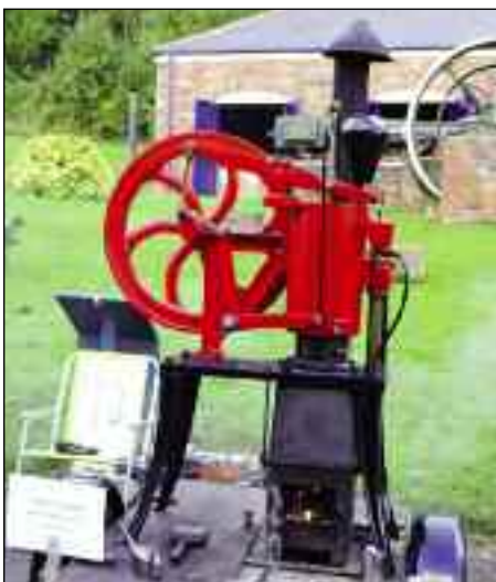
Stirling engine manufactured by Hayward-Tyler Ltd of Luton, 1898, to the Rider-Ericsson patent. Owned by Aubrey Burge of Pewsey in Wiltshire.
