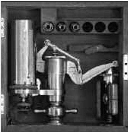
An engine indicator, assumed from manufacturing details to have been the work of Hannan & Buchanan of Glasgow c. 1890, displays RICHARDS PATENT NO. 10411. But there are obvious problems, as the relevant patent was actually no. 1450 of 1862. Had the indicator been made by the principal licensee, Elliott Brothers, it would be the 10411th made under the terms of the original licence (and made c. 1877). It is more likely to have borne a number linked to Hannan & Buchanan's order-book.
