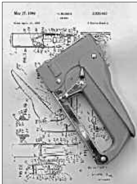
An accompanying invoice showed that this U.S.-made Swingline stapler had been purchased in 1981. However, the acknowledgement of two U.S. Patents indicate dates of 1960 and 1965. The later date is, therefore, the earliest the tool could have been made. Acquiring a copy of the older patent revealed the name of the inventor.
