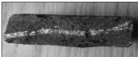
Fracture in wrought iron sample showing brittle layer
