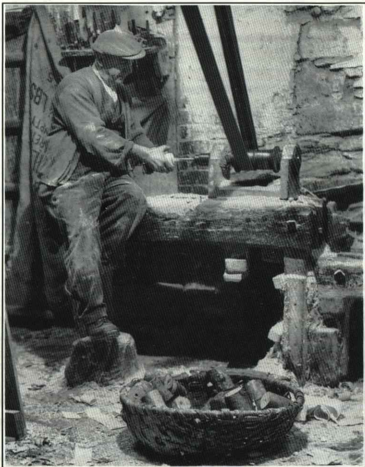
15.9: Stott Park top right: Steam engine in the bobbin mill right: Bobbin making, using the dangerous looking boring machine, the 'Rincer'
