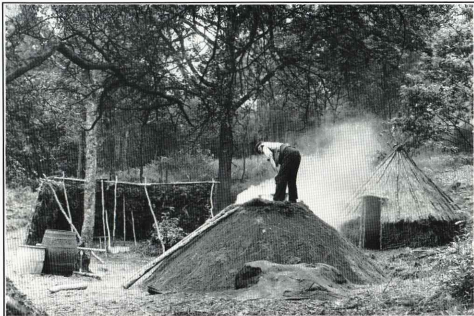
Traditional charcoal burning: Jack Allonby ensures that all is in order before the stack is sealed Photo: D W Jones
