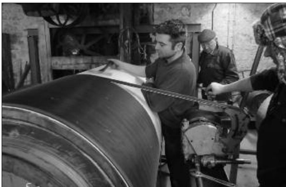
Knockando Mill – winding the new card cloth onto the drum
