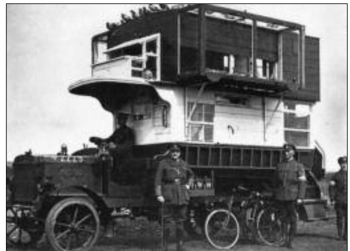
AEC 'B' Type converted to mobile pigeon loft during World War I
