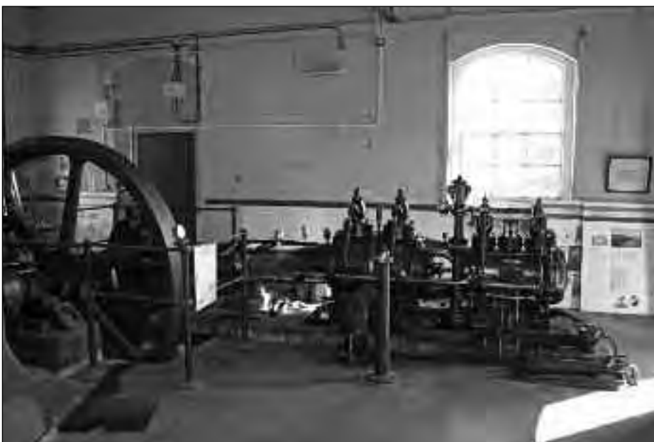
The Marshall class L 100 hp horizontal compound pumping engine at Owston Ferry
