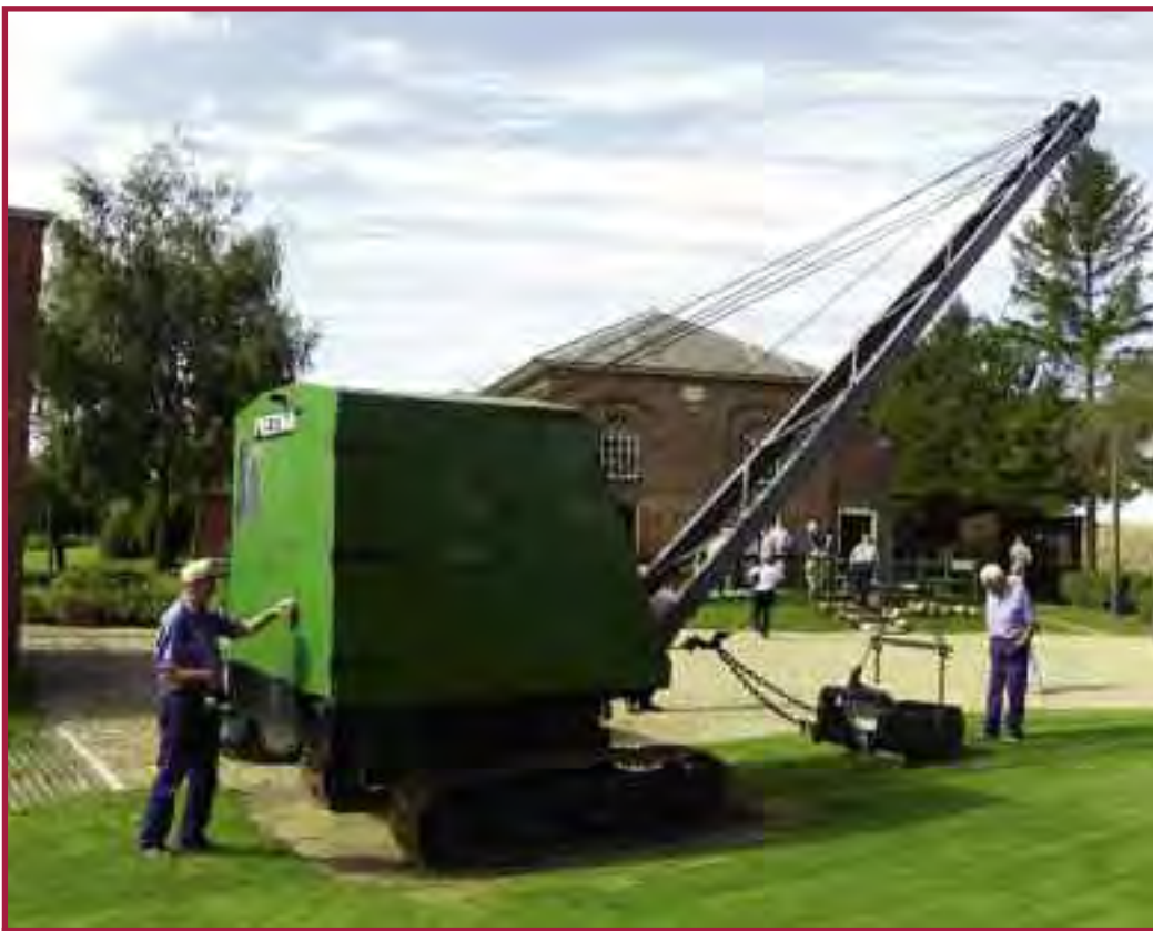
A Priestman excavator used for clearing fenland drains at Pinchbeck Marsh pumping station. See inside, page 2
