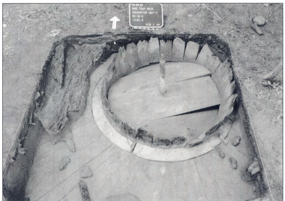
Detail of circular buddle centre, Ohio Trap Rock mine, Michigan, excavated in August 1995
