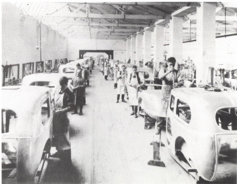
Car production in small brick and timber sheds. The SS, later Jaguar, car factory in a shell-filling factory erected during the First World War, Holbrook Lane, Coventry
