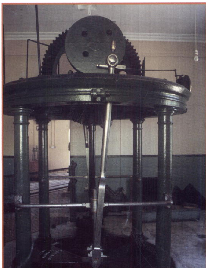
Water turbine pump of 1857 at the water museum at Sutton Poyntz near Weymouth, one of Dorset's best kept industrial secrets featured in a forthcoming day event (see Diary above) Photo: Peter Stanier
