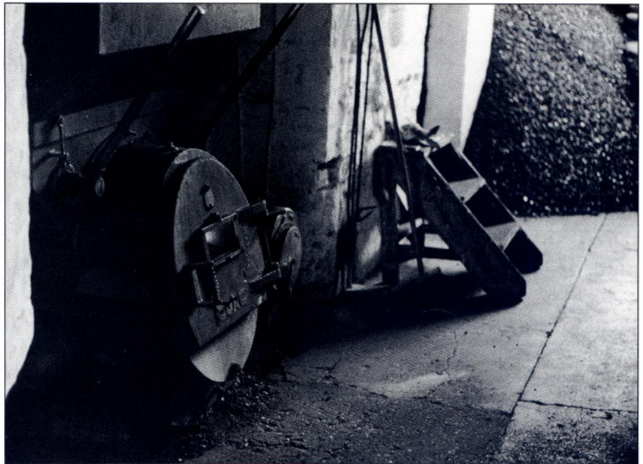
One of the Suxé anthracite furnaces at East Dereham maltings
