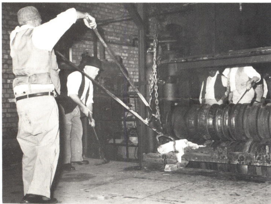
The 'backer' lifts a bloom (which is being reduced to 2½" square) during the demonstration run for Prince Charles. All the workers are ex - Walmsley and technical advice (for this caption too) was provided by Keith Gale.
