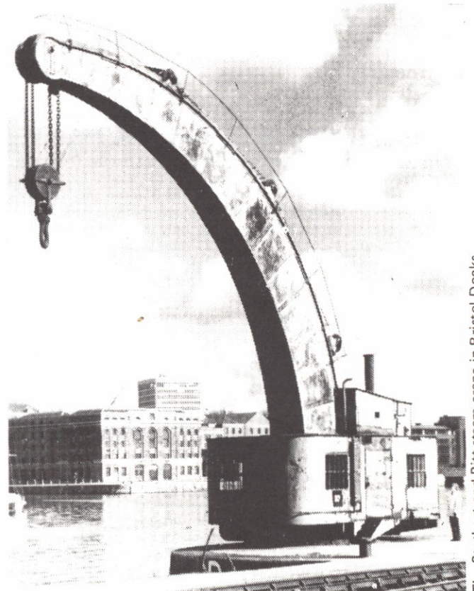
The Stothert and Pitt steam crane in Bristol Docks.
