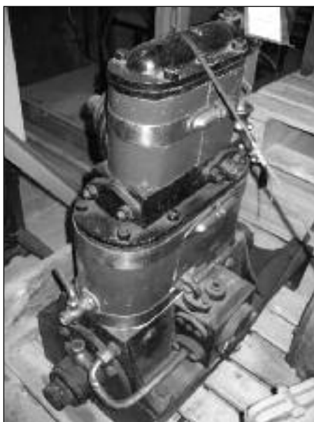
Willans design Hunter & English Three cylinder steam engine, now in the Birmingham Museum Collection Centre
