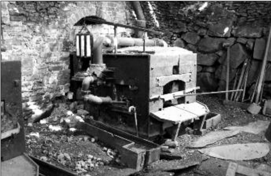
Lancashire forge at Engelsberg. This used an adaptation of the 'puddling' process to suit charcoal
