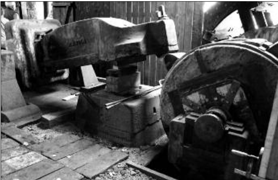
Trip hammer at Trångfors to work the iron into bar. Last used in 1919
