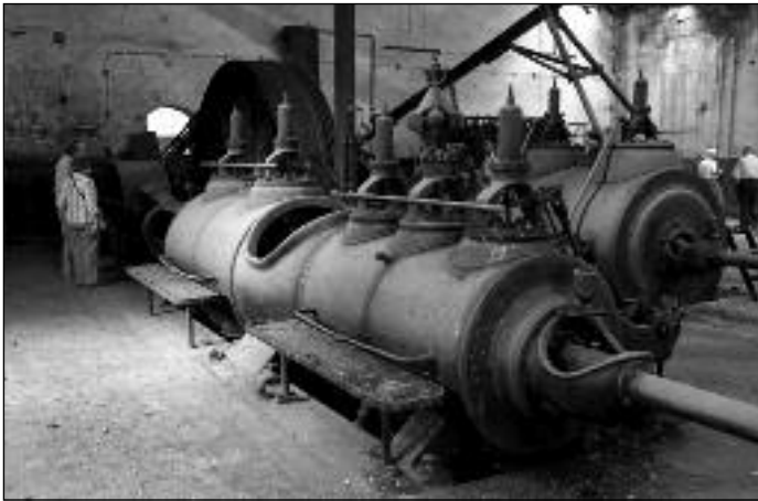
Triple expansion cross compound Sulzer
