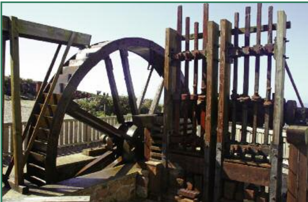
The waterpowered Nanchedra tin stamps on display at the Geevor Mine in west Cornwall. See inside, page 5.
