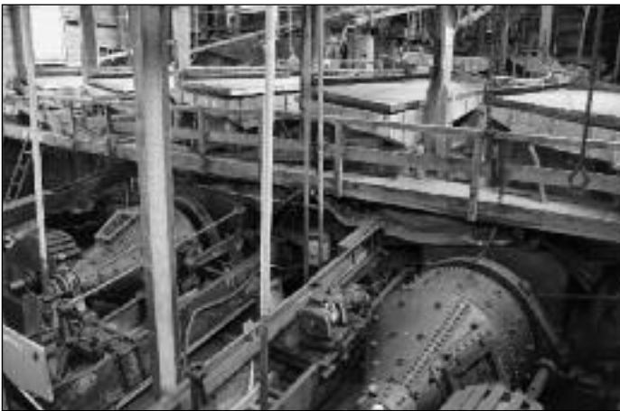
Ball mills and shaking tables in the dressing mill at Geevor Mine
