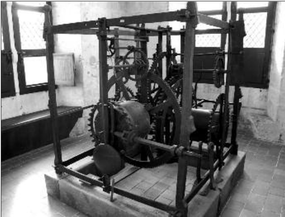
Mechanism of the medieval Gros Horloge (Great Clock) in Rouen
