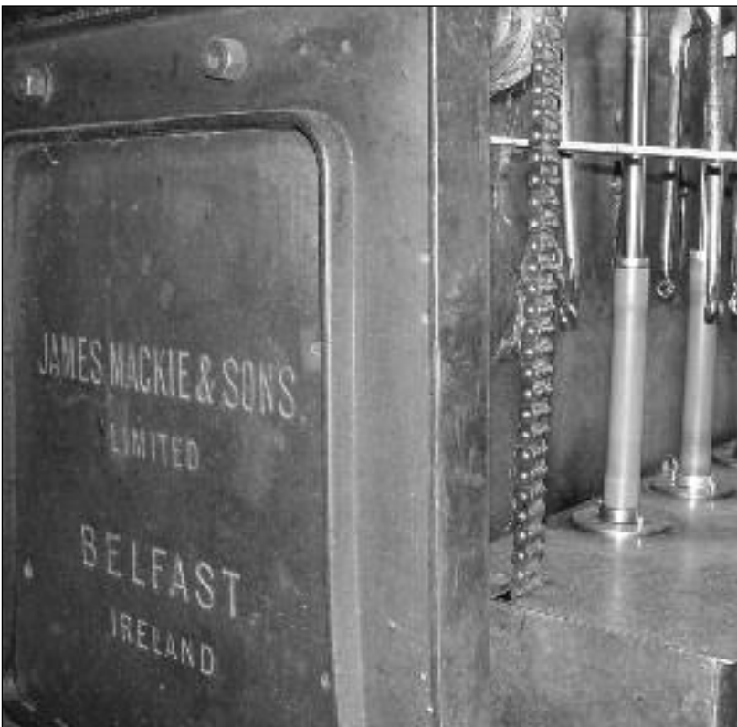
Roving frame by James Mackie of Belfast in the Orzel flax mill, Lower Silesia, Poland
