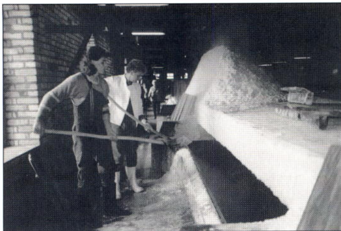
Workers shovelling salt from steaming supersaturated brine at Ciechocinek
