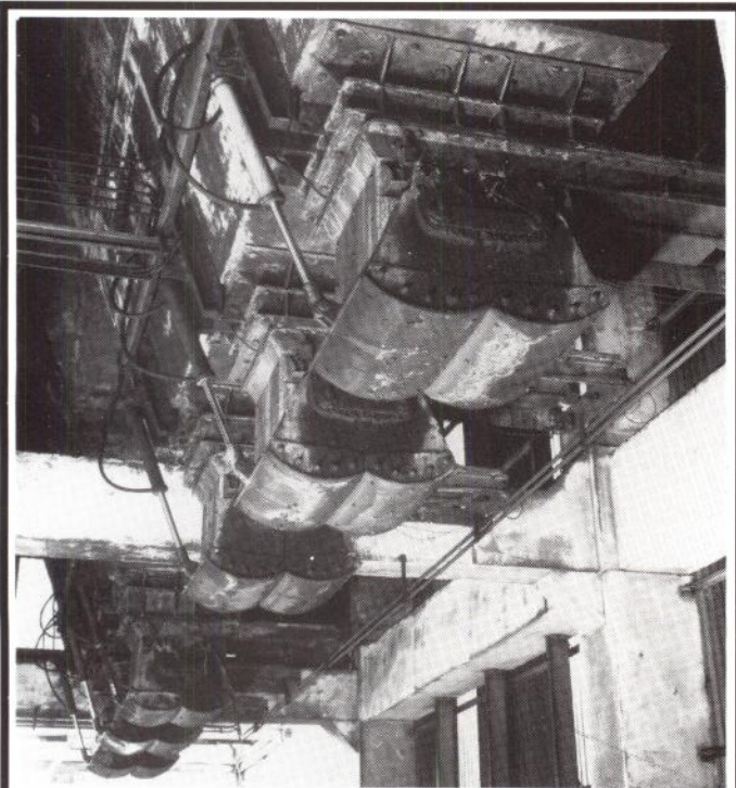
Colliery recording in Wales, October 1992: an underside view of hydraulically operated doors of the rapid rail loading bunkers at Taff Merthyr Colliery, Mid Glamorgan, which closed last year and is under demolition. There are three glass-lined bunkers, with a combined capacity of 2,000 tonnes of coal, and each 28-wagon train was loaded and weighed while on the move. Aberthaw Power Station near Barry took the entire output from the colliery at the rate of one 900 tonne train each day. This photograph is part of the survey of Taff Merthyr Colliery carried out by the Royal Commission on the Ancient and Historical Monuments of Wales, is in preparation for the Commission's forthcoming publications on collieries. The first of these is due for distribution through Alan Sutton Publishing later this year, Colliery Architecture and Engineering in Wales.
