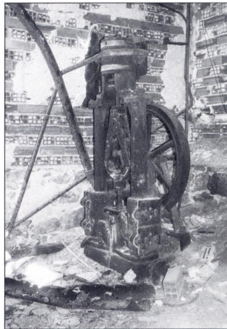
Vertical steam engine, originally built as a pump and here employed to drive a generator Photo: Paul Vigor
