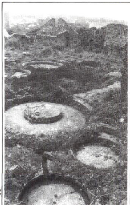
2. Concrete centre-head buddle, West Basset, Cornwall, 1875
