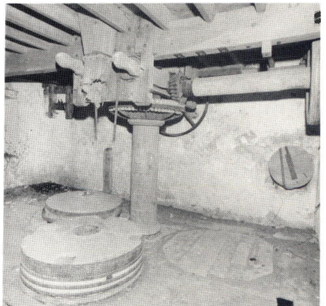
Part of a completed NMR Survey: King's Mill, Pembrokeshire. Exterior view of mill, house and cartshed. Interior view layshaft bearings and crown wheel.
